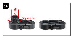
To use Pole 1 or Pole 2 upper unit on tripod adapter, the fitting must be installed. Loosen the side knob. With the flange facing up, squeeze and push the fitting into the adapter. The fitting should snap in place. Then continue to **Step 6**.
