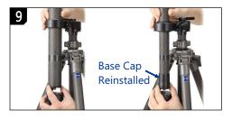
Slowly lower the pole while holding the base with one hand. Twist the upper adapter to align for the 3/8" thread on the rotator. Then carefully tighten the pole to the rotator. When a motorized rotator is used, skip this step and go to **Step 9A**.
