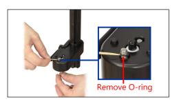
The screws are made captive by using rubber O-rings. If only one type of screw will be used, the unused one(s) can be removed. Simply pull the M6 screw knob downward to remove it. Use a hex key to push the M5 screw up. Use a toothpick or similar to remove the O-ring. Then the screw will come off with hex key.
